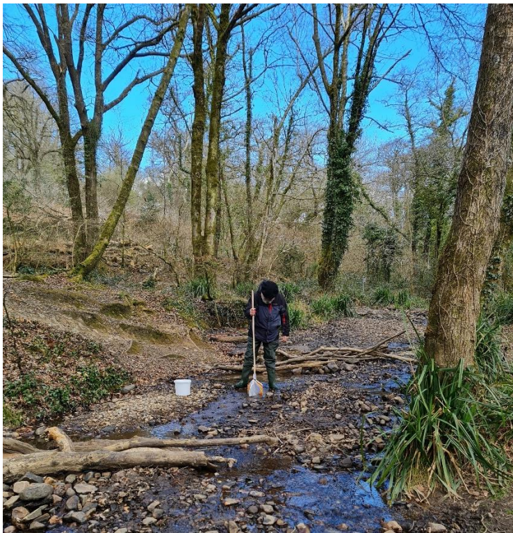
Figure 3 Sample collection at the entrance of pond using kick sampling method.
