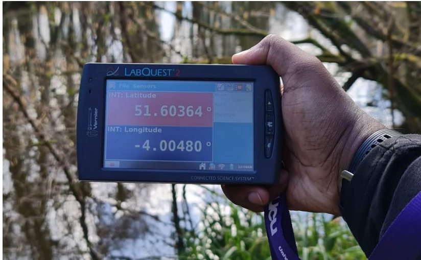
Figure 2 Collecting field data using the LabQuest2 data collection equipment
