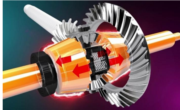
Figure 8: Cone Clutch LSD, (Left) Construction (Stone & Ball, 2004), (Right) Operation (Autodata Training, 2019).
