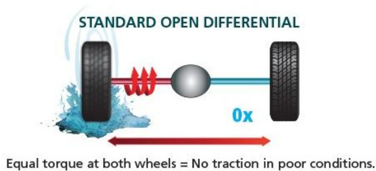
Figure 3: Open Differential (Top) Components (Crouse & Anglin, 1983), (Bottom) Traction Problem (AuburnGear, n.d.).
