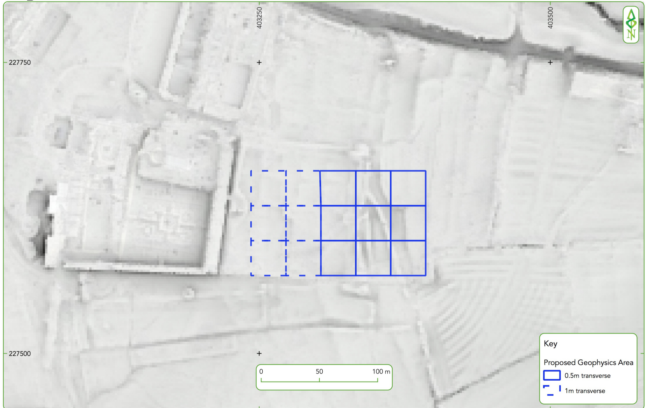
Figure 4. Proposed area for earth resistivity geophysical survey divided into 30m x 30m grids
