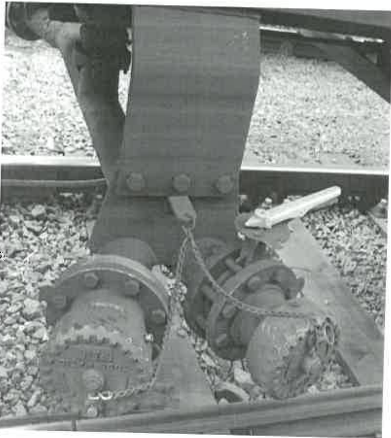
Figure 5 – Indicates the handbrake on the dedicated rail car being loaded or transported.
