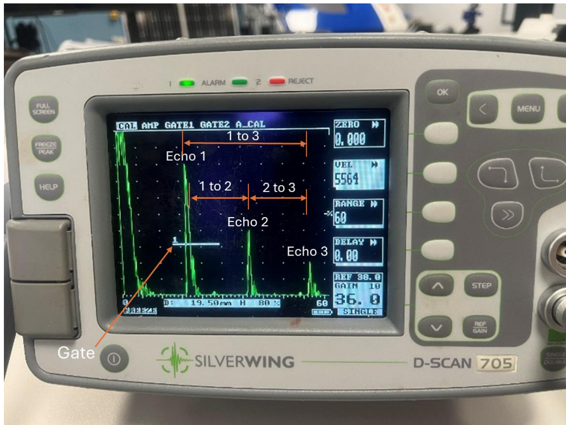
Figure 2 - Wave amplitudes for mild steel block with annotations
