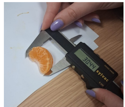
Image 1: Length measurement taken with electronic callipers (Dabell, 2026a)
