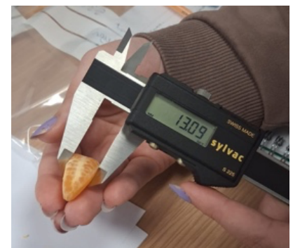
Image 2: Width measurement taken with electronic callipers (Dabell, 2026b)
