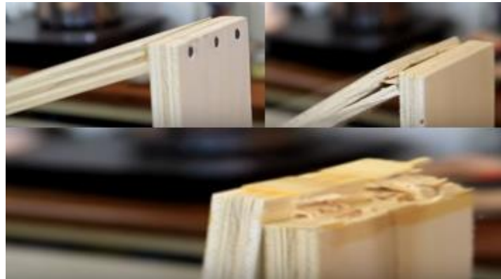
Figure 10 - end screws top left then pocket top right then dovetail
