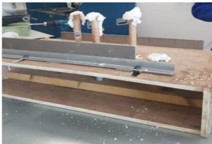
Figure 11 - clamp dowels and expanding foam.
