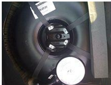
Autogas tank inside spare wheel recess
