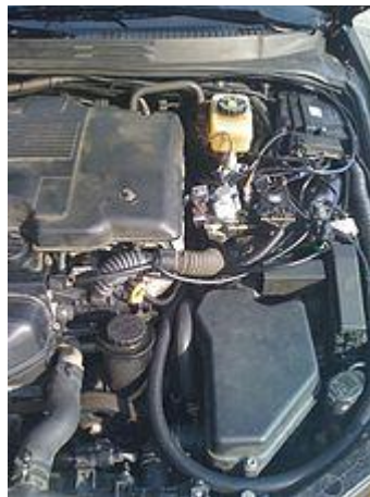
Vialle LPI liquid injection on a 2003 Lexus IS 300 2JZ-GE.
