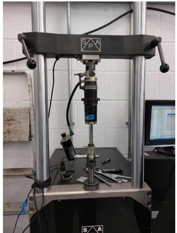
Figure 6 - Damper Curve Investigation
