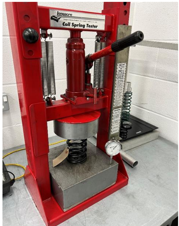
Figure 4 - Spring Stiffness Investigation
