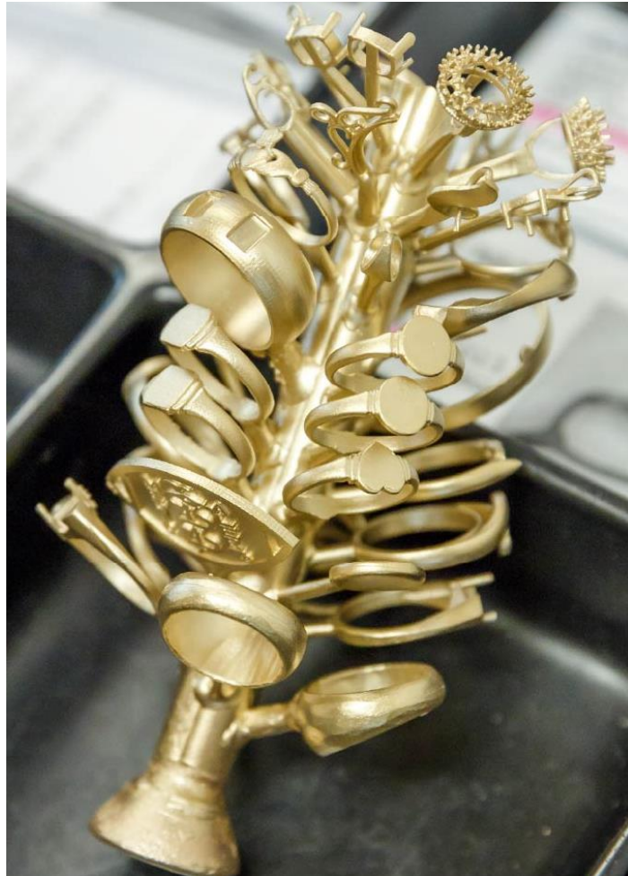
Figure 6 - A yellow gold casting tree. (Morris and Watson)
