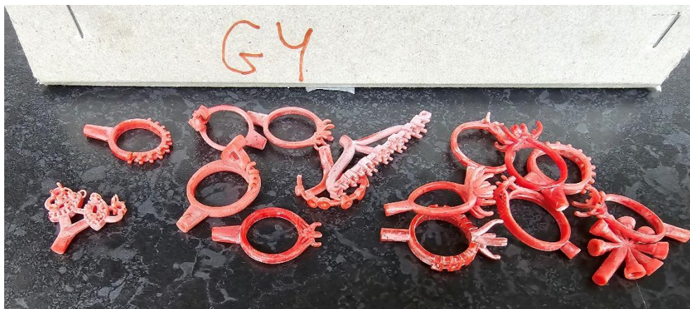
Figure 8 - A collection of defected Visijet Wax Jewel Red models about to be put into the wax GY (graveyard)
