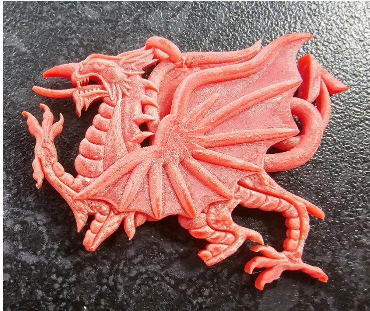
Figure 9 - Visijet Wax Jewel Red model deformed by being dropped on the floor
