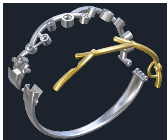
Figure 2 - The bangle in Figure 2 shown in 3Design split into separate parts for 3D printing and precious metal casting.
