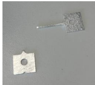
Figure 7 – Aluminium sample post testing after experiencing failure.
