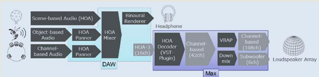
Fig. 5. Overview of the audio system during the production phase of the large-scale 3D audio-visual installation shown in Fig. 4. The DAW and Max are running on two separate PCs, respectively. The purple and red dots represent the loudspeakers and subwoofers positions, respectively.
