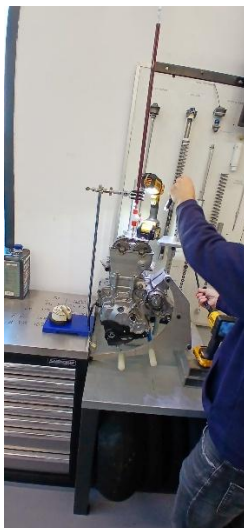
Figure 2-3- Clearance Volume verification experiment.
