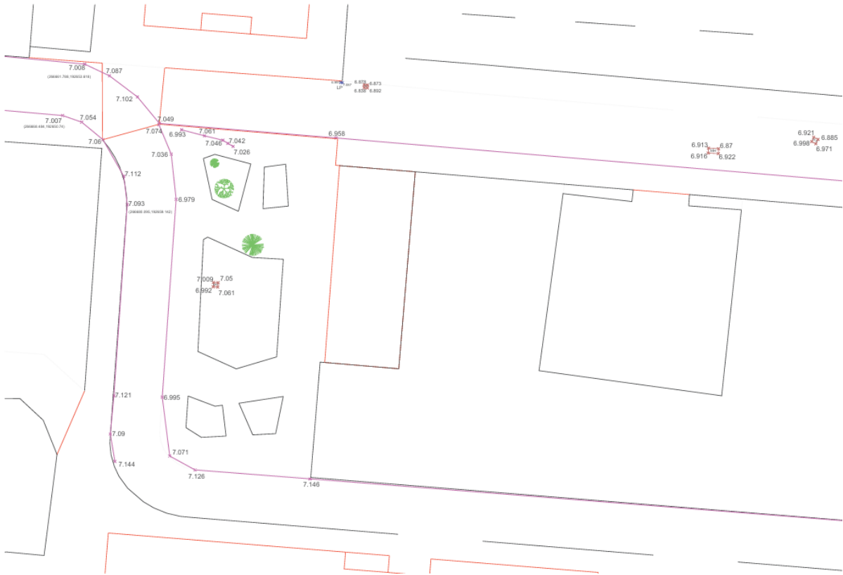
Figure 3: Screenshot of captured spot coordinates imported into AutoCAD and overlaid on an Ordnance survey base map.
