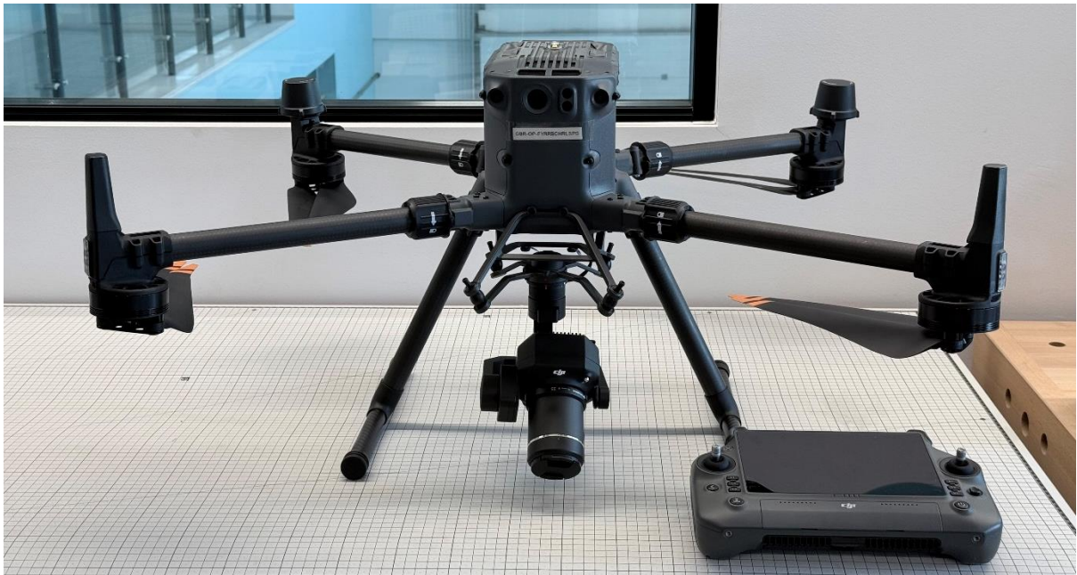
Figure 4: Drone used to capture images used in the production of a photogrammetry derived point cloud.
