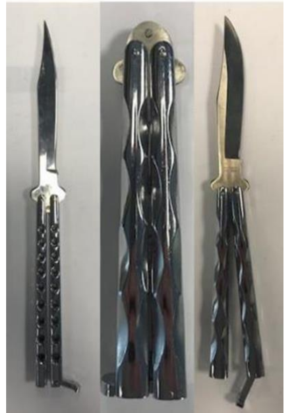
Note the manual locking point at the bottom to secure the two handles together.
