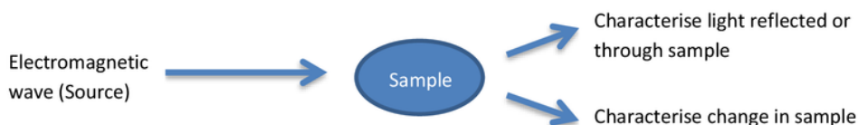
Figure 2 – Diagram showing basic principles of spectroscopy
