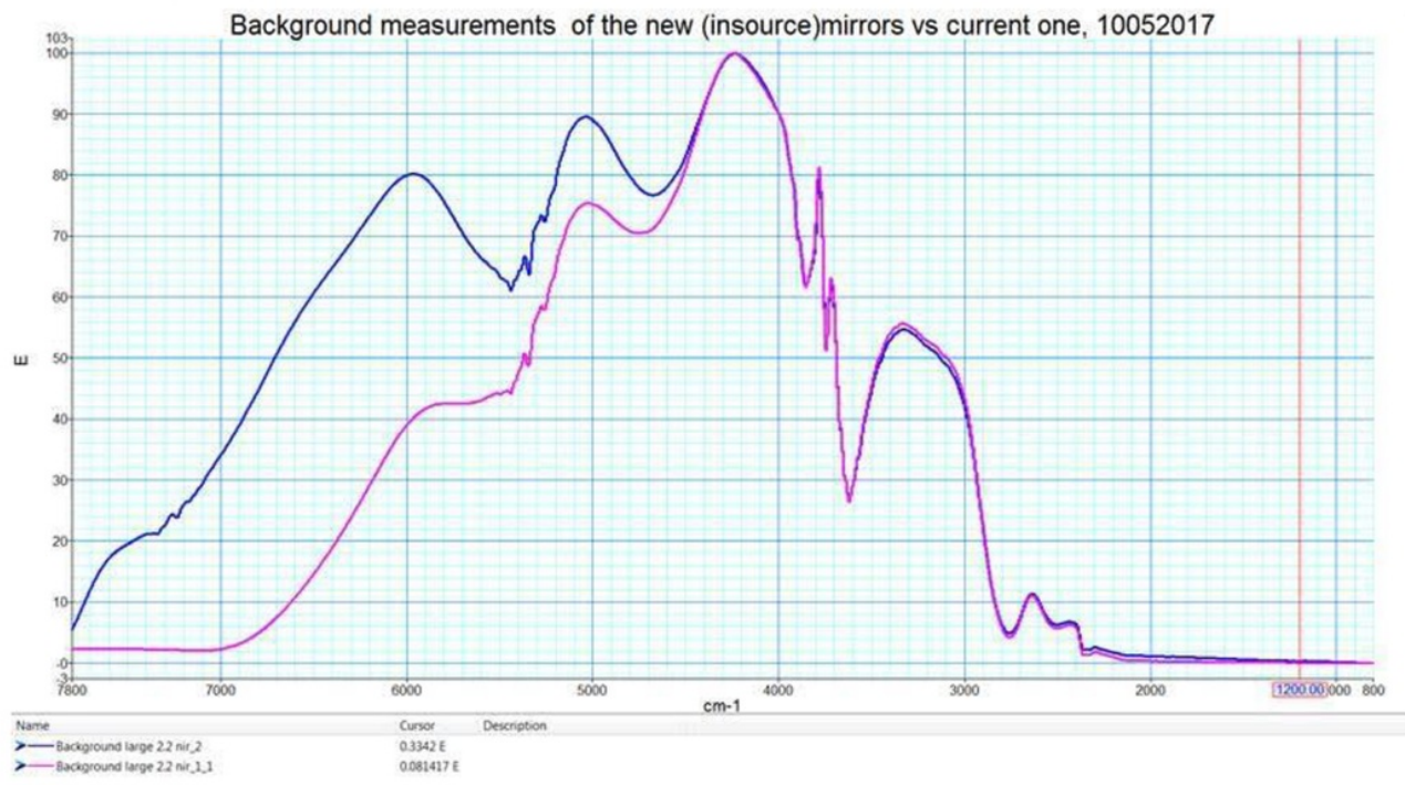
Figure 10 Reflectance of Dichroics Old and New (PerkinElmer, 2018)
