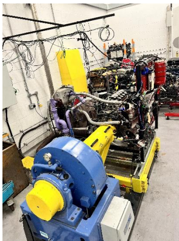
Figure 2-shows the Schenck dynamometer attached to the Honda engine.
