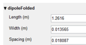
Figure 5: Folded dipole dimensions
