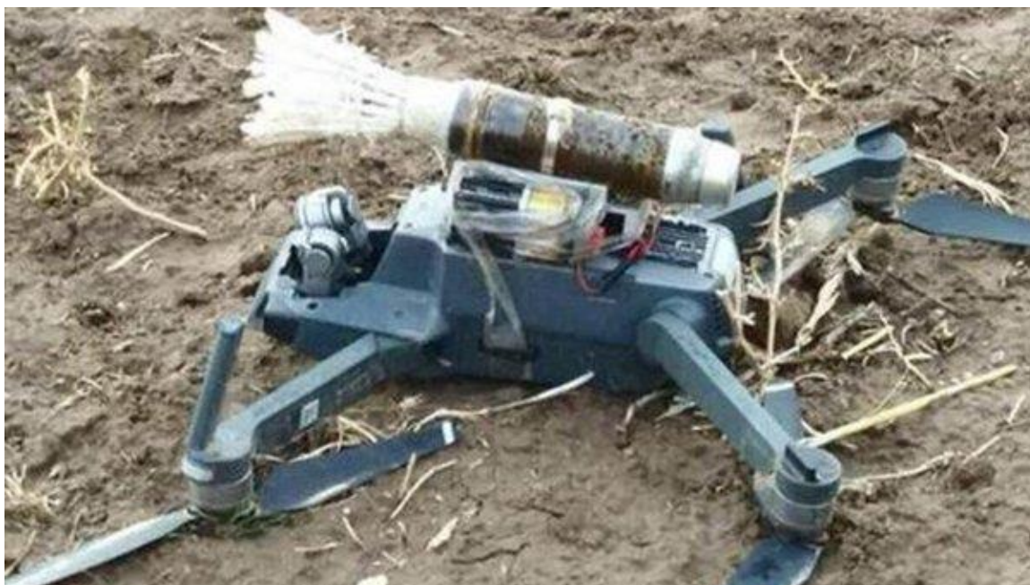
VOG 17 Rifle grenade dropped from a drone
