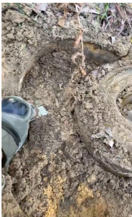
ML-8 located under a TM 62 M Mine
