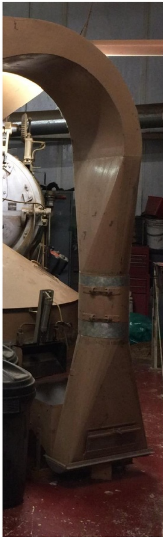
Figure 9: The exit door from the paddle. Figure 10: The riser from the paddle to filling section of the process.
