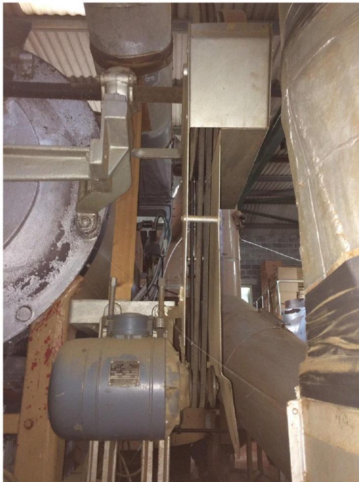
Figure 7: The motor pulley system used to rotate the roasting drum.
