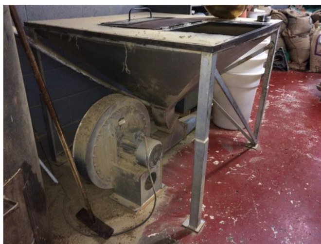
Figure 2: The hopper and blower for the raw beans, the start of the process.
