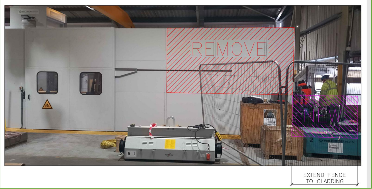
Tool Changing Trolley and Mods to Guarding to allow reduced movements of Tooling
