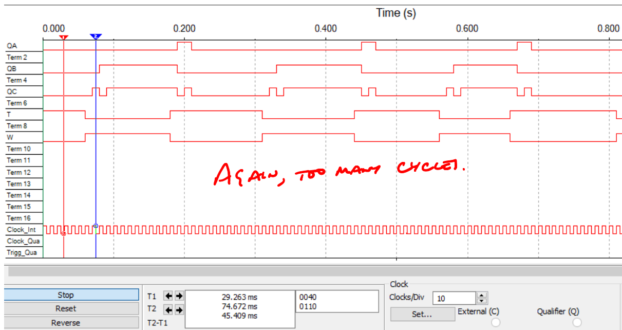
Figure 11: Logic analyser testing green traffic light (state 0).
