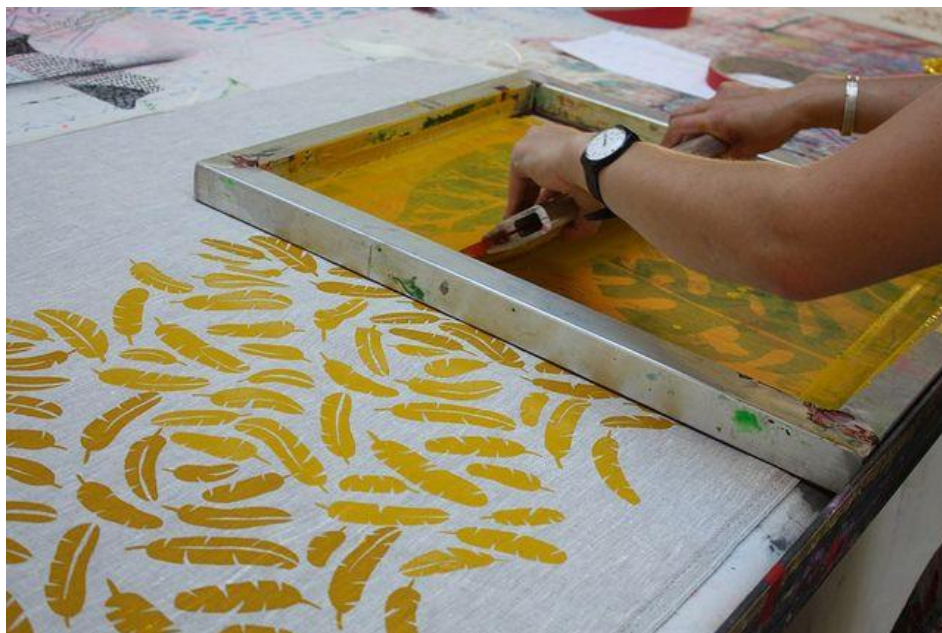
Figure 1 Hand screen printed textile
