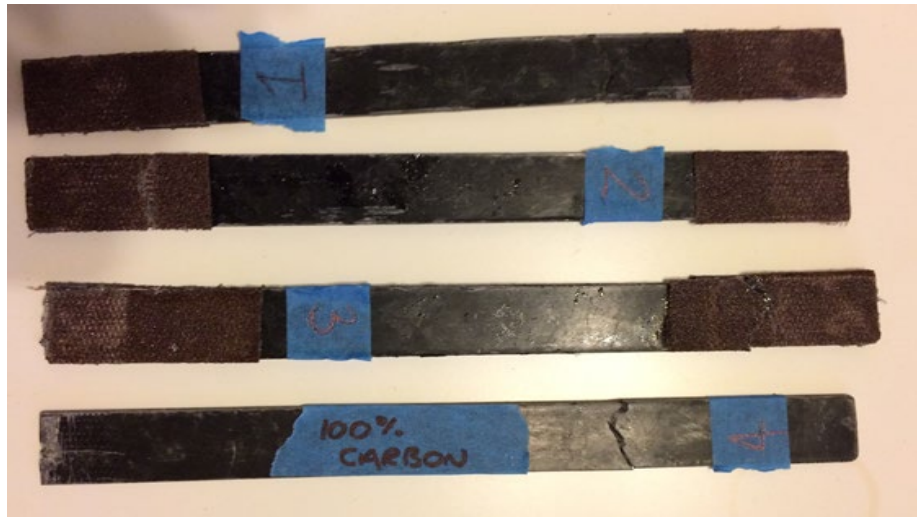
Figure 5 CFRP Specimens After the Tensile Test Experiment.
