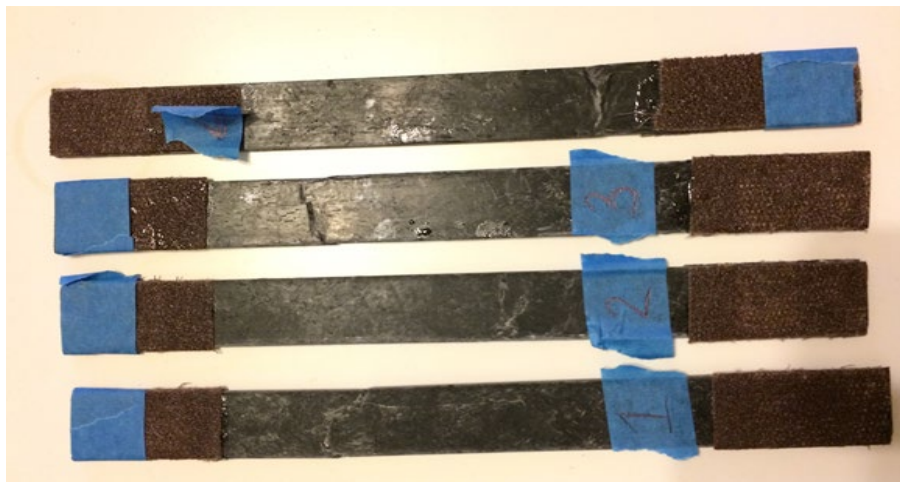
Figure 4 GFRP Specimens After the Tensile Test Experiment.
