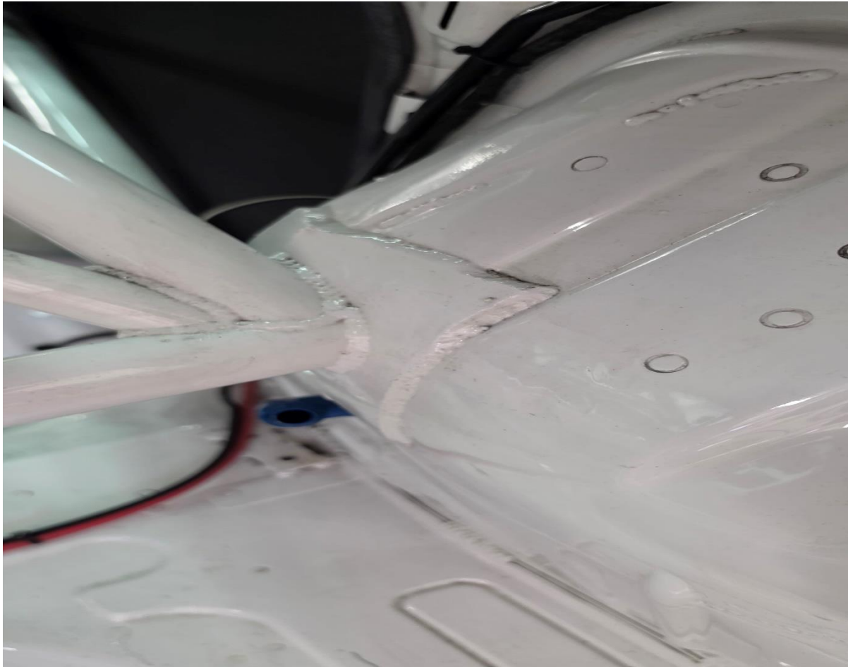
FIGURE 2: CLOSE-UP OF WELDED JOINT SHOWING HEAT-AFFECTED ZONE (UWTSD WORKSHOP)
