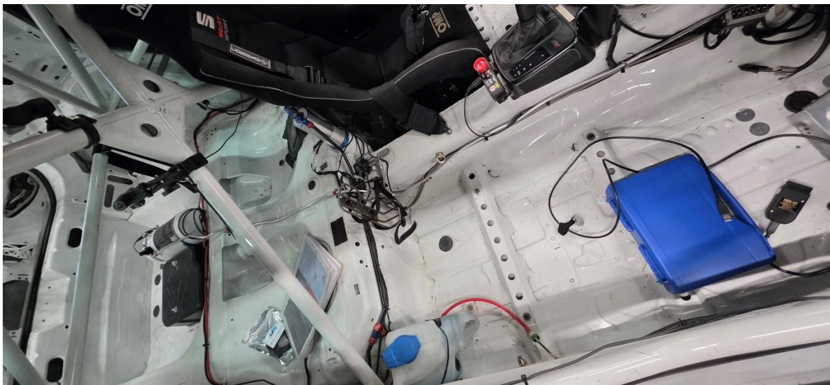
FIGURE 1: INTERIOR VIEW SHOWING INTEGRATED ROLL CAGE AND STRIPPED BIW STRUCTURE (UWTSD WORKSHOP)
