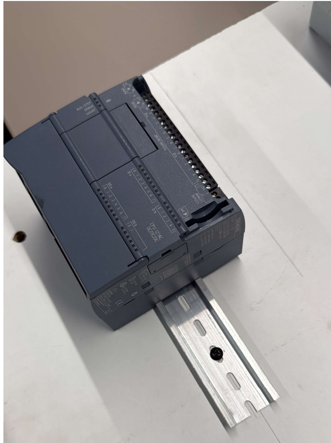
Figure 126 - PLC mounted to din rail
