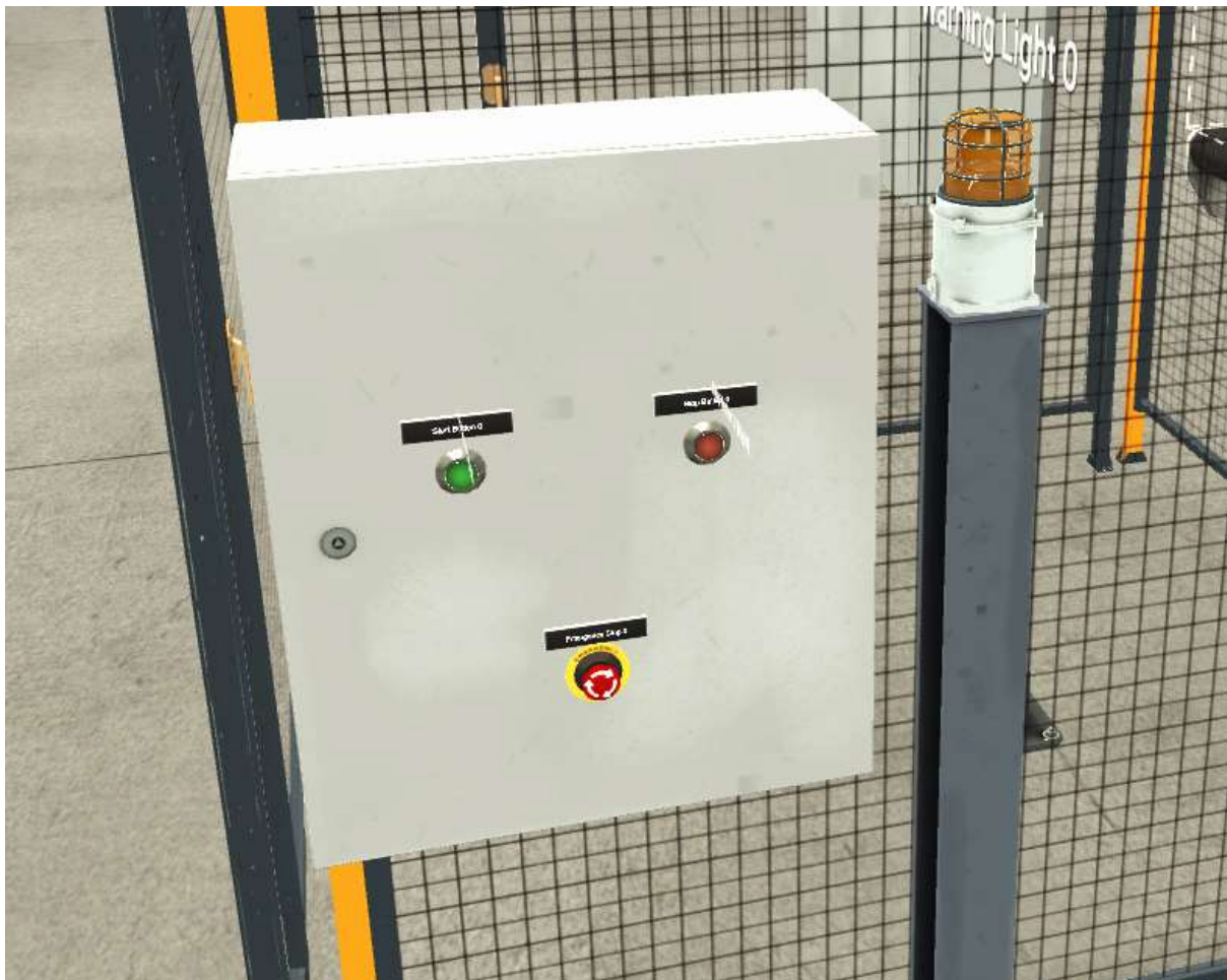
Figure 122 - Control panel and signal light
