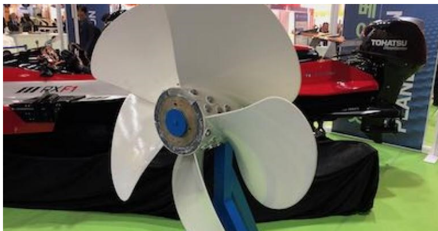
Figure 6 – CRP propellor with removeable blades for ease of maintenance
