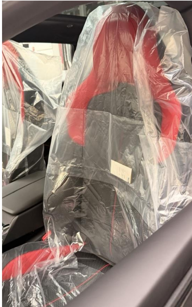
Figure 3 - Seat Protective Cover Fitted During Production
