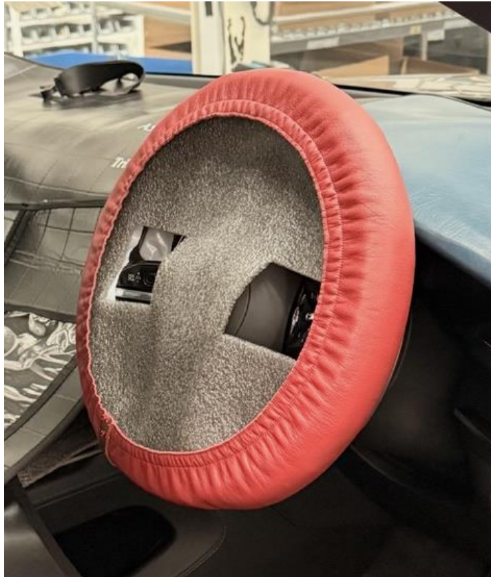
Figure 5 - Steering Wheel Protective Cover Fitted During Production
