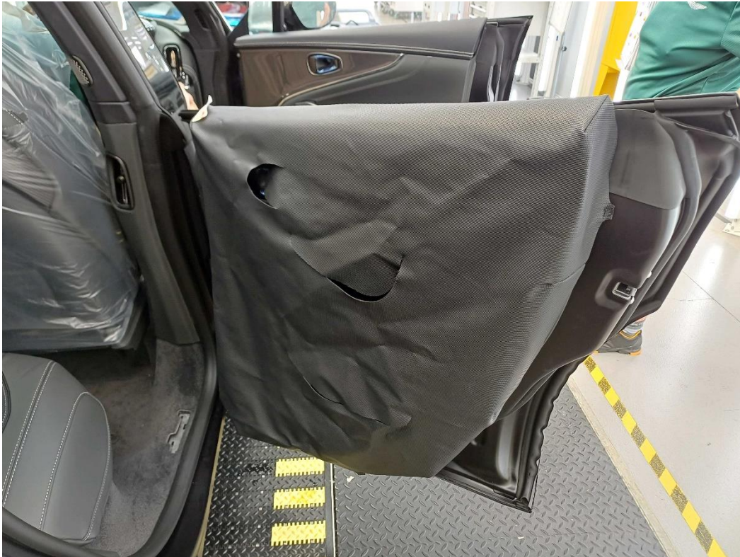
Figure 8 - Door Card Protective Cover Fitted During Production
