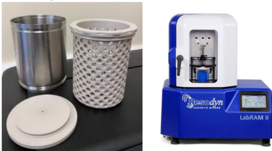
Figure 4 - TFP Milling Vessel, Cage and a Resodyn LabRAM II
