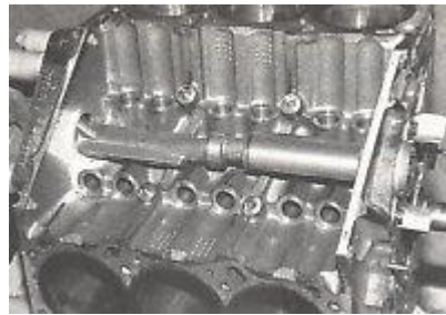
Single balancer shaft inside the V-valley
