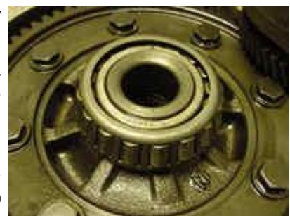
A tapered roller bearing from a manual transmission
