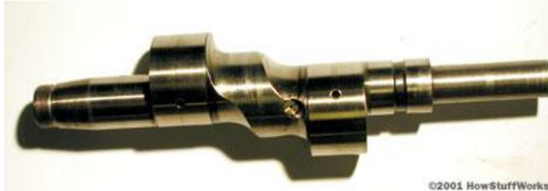
The output shaft -- note the eccentric lobes
