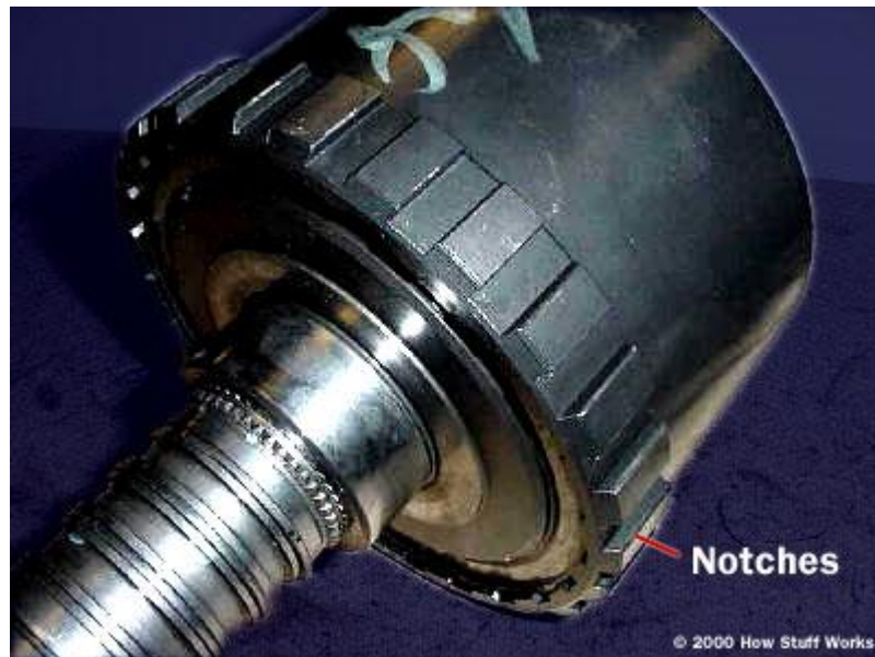
Figure 11 The output of the transmission The square notches are engaged by the parking-brake mechanism to hold the car still.
