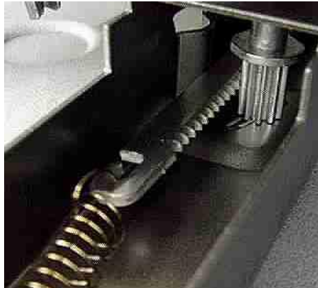
Figure 9. Rack and pinion gears from a household scale
