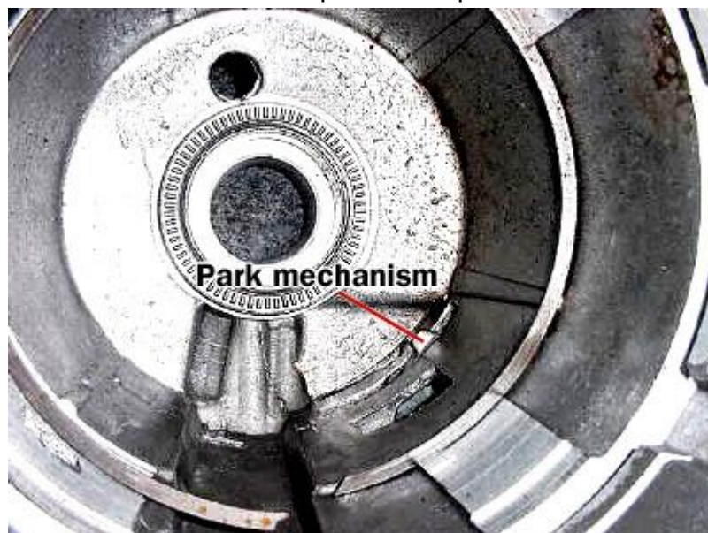
Figure 12 The empty housing of the transmission with the parking brake mechanism poking through, as it does when the car is in park
