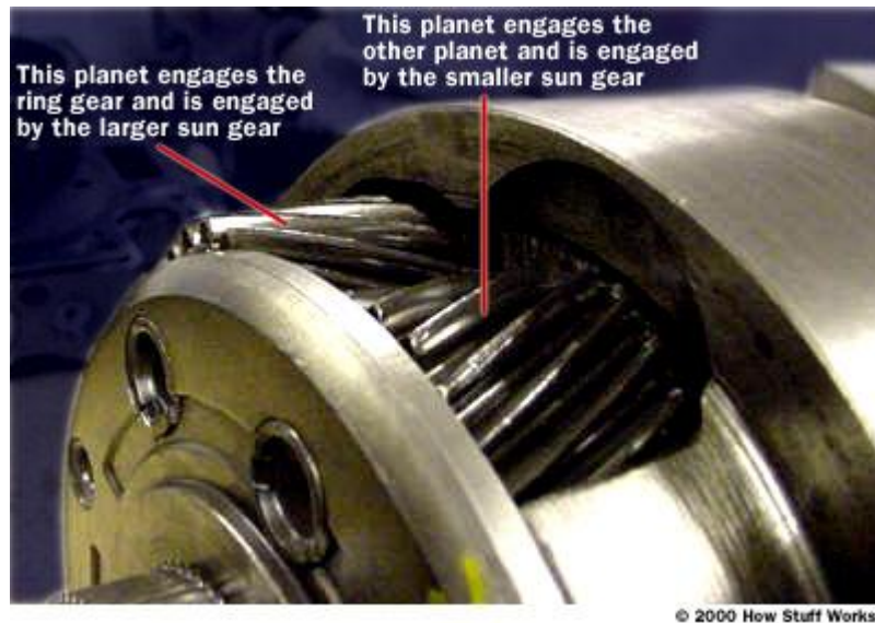
Figure 4 Planet carrier: Note the two sets of planets.
