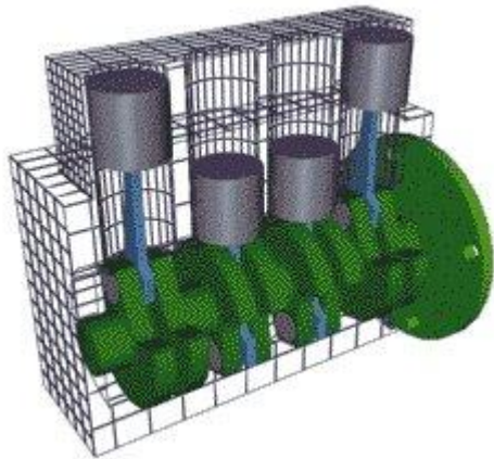
Figure 2. Inline -- the cylinders are arranged in a line in a single bank.
