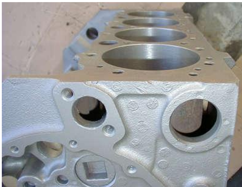
Note that the walls of the cylinder are quite thin, and that the engine block is mostly hollow.
