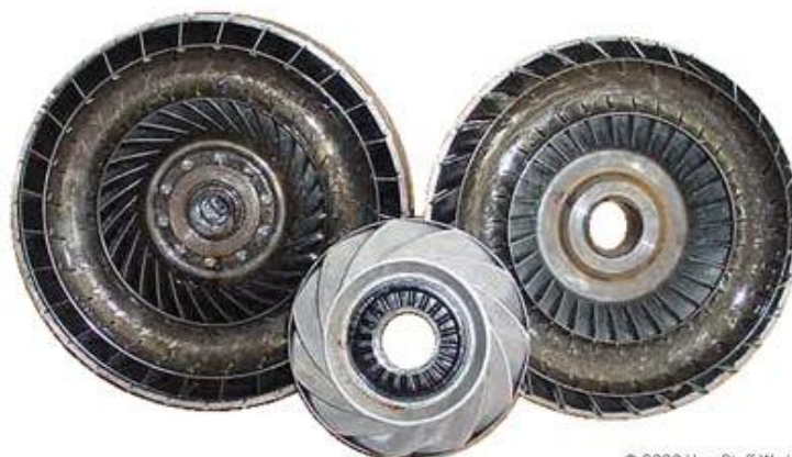
The parts of a torque converter (left to right): turbine, stator and pump
