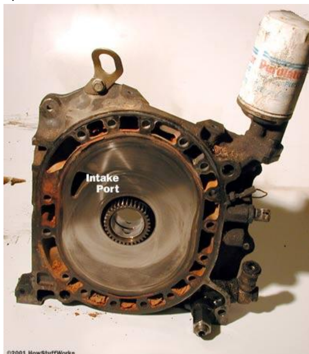
One of the two end pieces of a two-rotor Wankel engine
