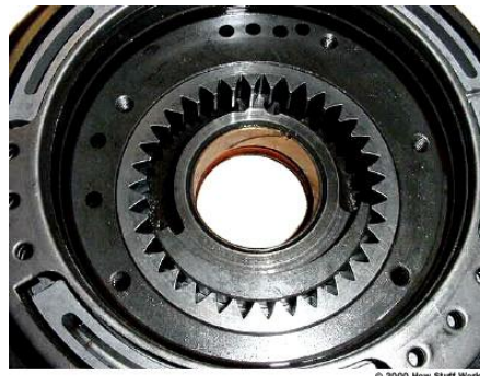
Figure 16 Gear pump from an automatic transmission
