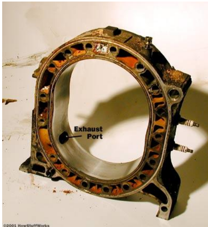
The part of the rotor housing that holds the rotors -- note the exhaust port location
