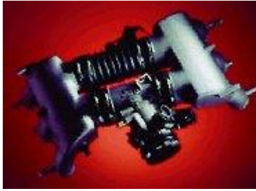
Porsche 996 GT3's resonance intake system. Note that 2 pipes connect between the 2 plenums.
