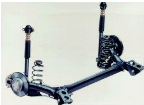
Golf's torsion beam rear suspension
