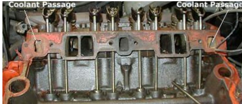
The head of the engine also has large coolant passageways.
