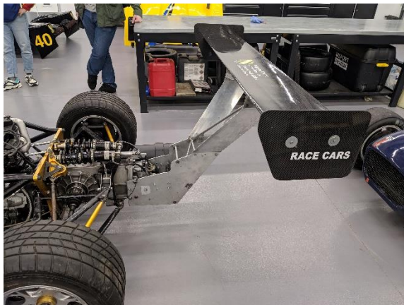
Figure 4.5.3 – The current SRCC RA1 wing and mounting on the MCR chassis, along with a view of the profile.
