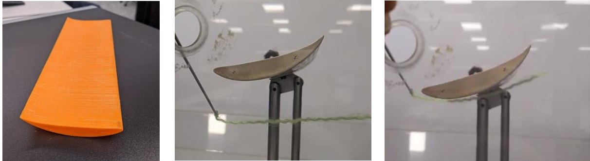
Figure 5.2.1 (a b c) – 3D printed scale model of the SRCC wing being tested in the wind tunnel at different angles of attack. In the right picture (c) separation can be seen to occur as the thread violently moves around in the turbulent air.
