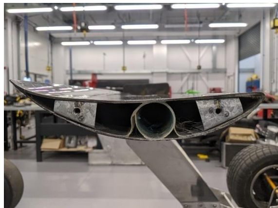
Figure 4.5.3 – The current SRCC RA1 wing and mounting on the MCR chassis, along with a view of the profile.
