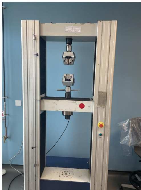
Figure 3- Denison Mayes tensile testing machine used for specimen testing
