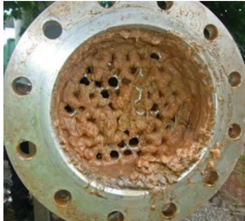
Figure 7 - Shell and Tube Heat Exchanger - Deposition Fouling - [20]
