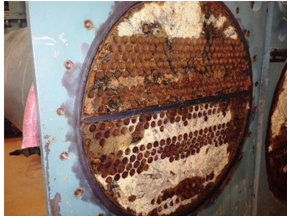
Figure 5 - Shell and Tube Heat Exchanger - Corrosive Fouling - [24]
