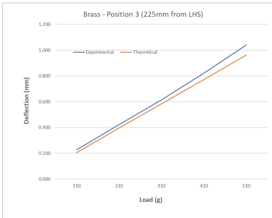
Figure 9 - Graph showing Load vs Deflection for Brass beam in position 3
