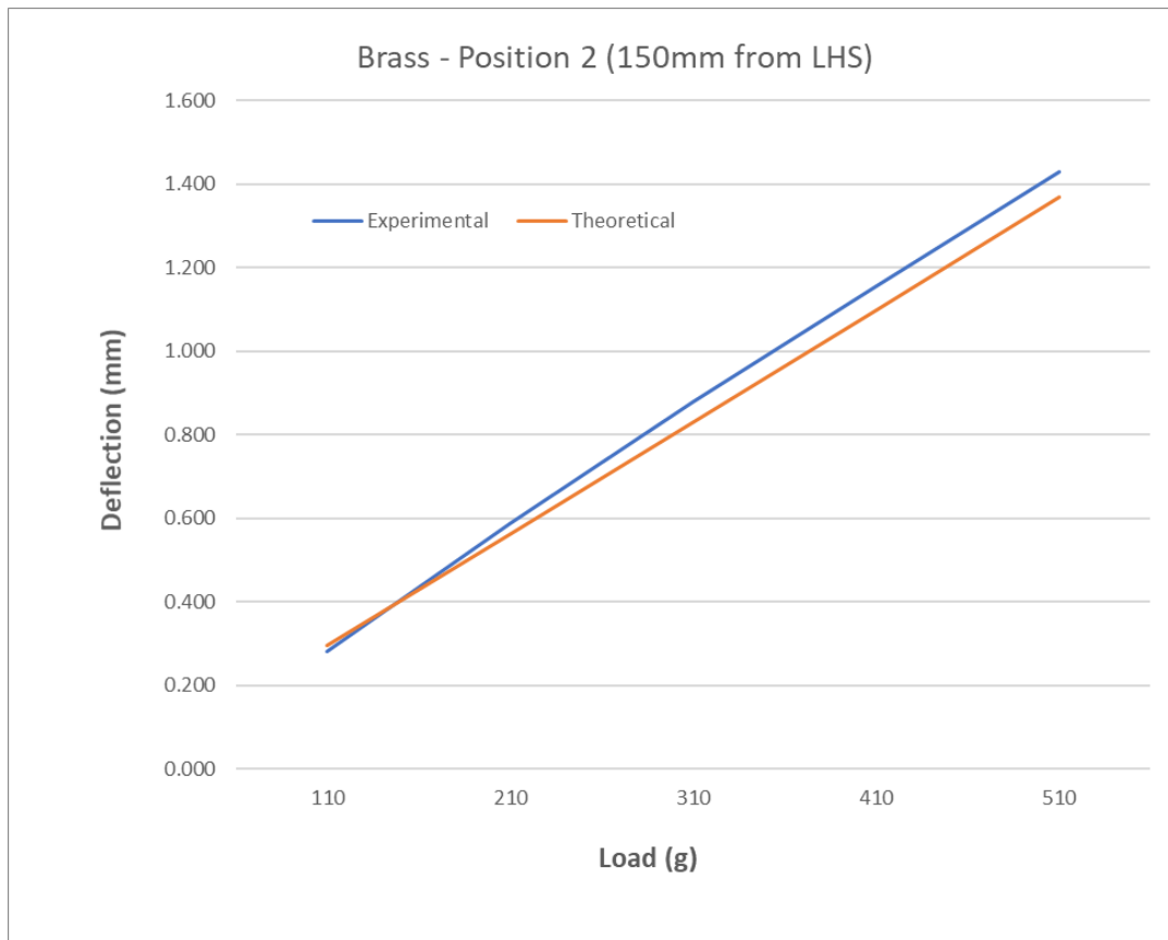
Figure 8 - Graph showing Load vs Deflection for Brass beam in position 2
