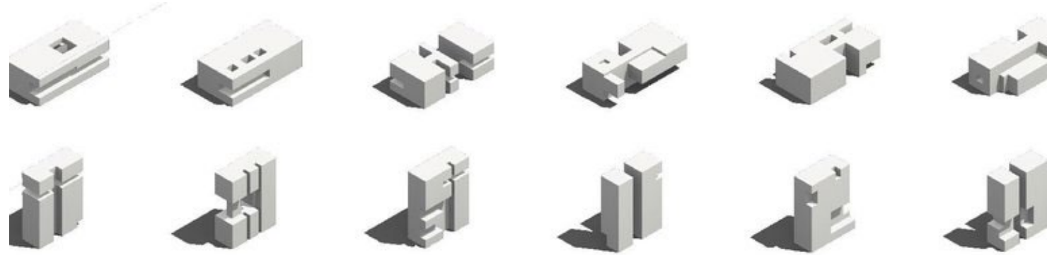
Building massing generation model based on the subtractive form generation principle
