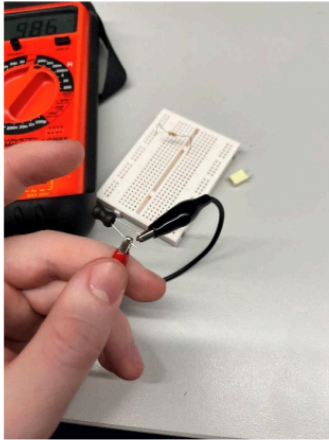
Figure 3: The inductor under test to find the components values
