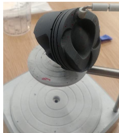
Figure 9-60: Piston Crown of the Ford Fox GTDI Engine in the Process of Surface Scanning
