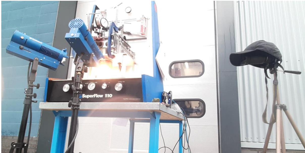
Figure 5-6: In-Cylinder Turbulence Visualization Experiment Setup
