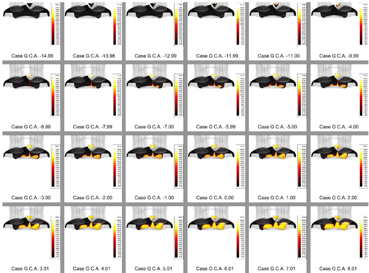
Figure 6-28: Case G Temperature Contour Front View
