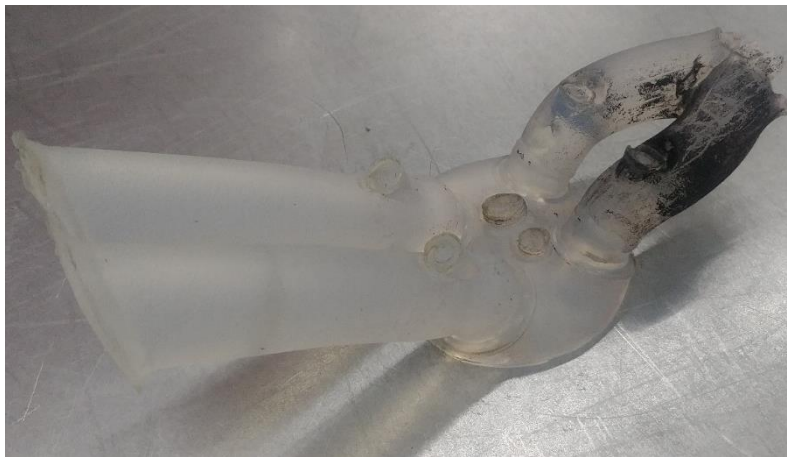
Figure 9-59: Single Piece Positive Volume Cast of Ports and Combustion Chamber of the Ford Fox GDI Engine
