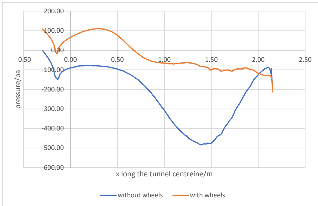
Figure 42 pressure distribution along the tunnel centreline
