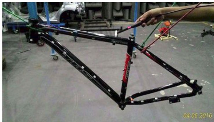
Figure 3 - EMA testing done on a mountain bike frame. (Sani, et al., 2016)
