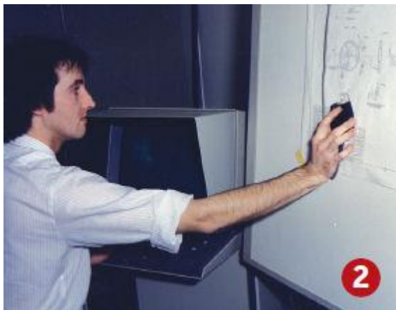
Figure 2- Image of a digitising tablet used to create a nodal mesh for FEA CAD integration. Source- (Abbey, 2013)
