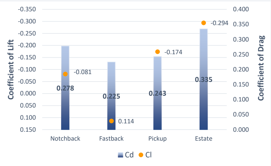
Figure 6 – MIRA Geometries Drag and Lift Coefficients. Drag Values are in bold.
