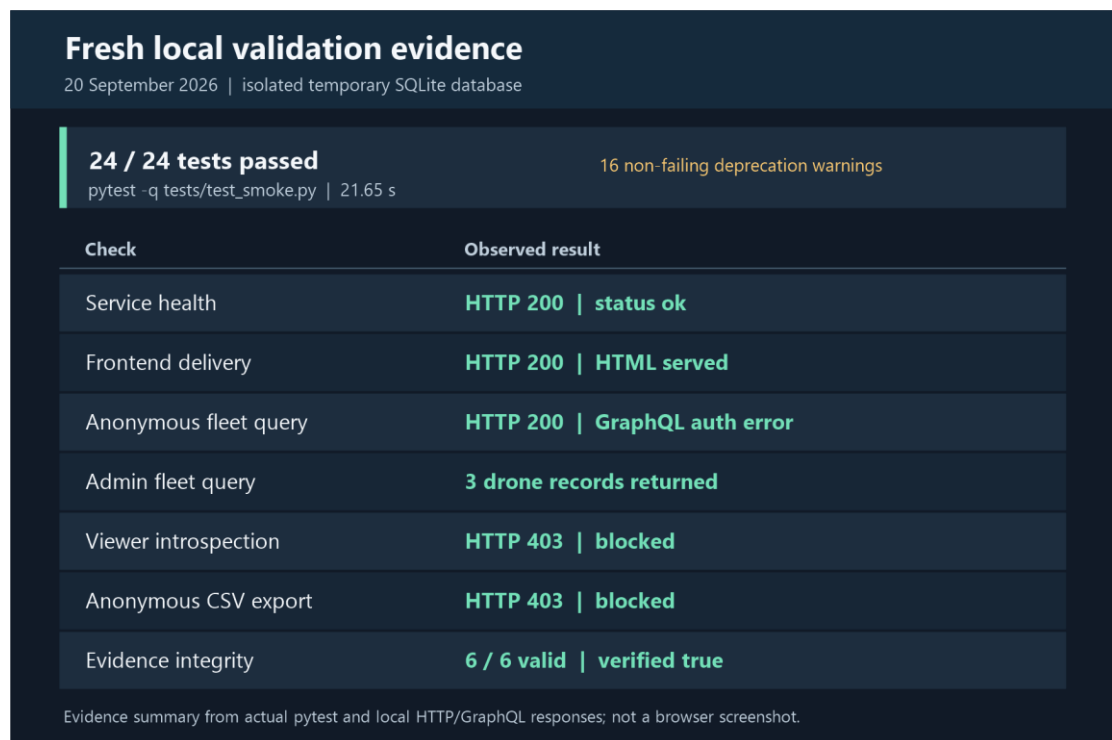
Figure A.1 Fresh isolated validation summary from actual pytest and live API responses (20 September 2026)
