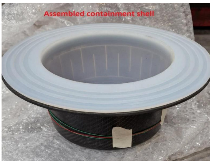
Figure 4 - Fully assembled containment shell with can protection feature
