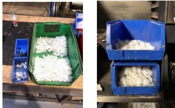
Figure 46: Two Bin System
