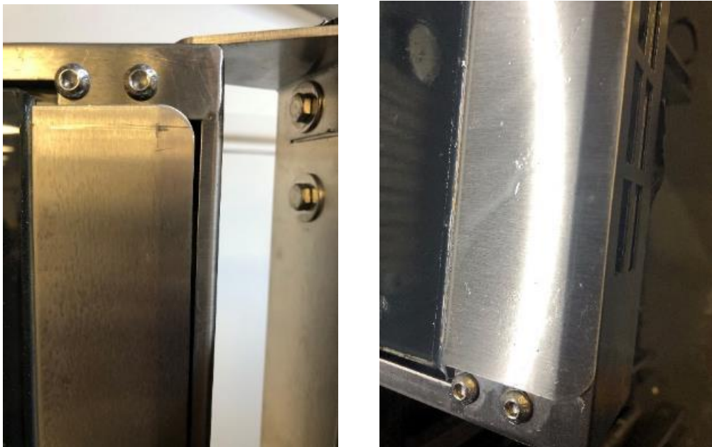
Figure 36:Oven Door Catching Issue
