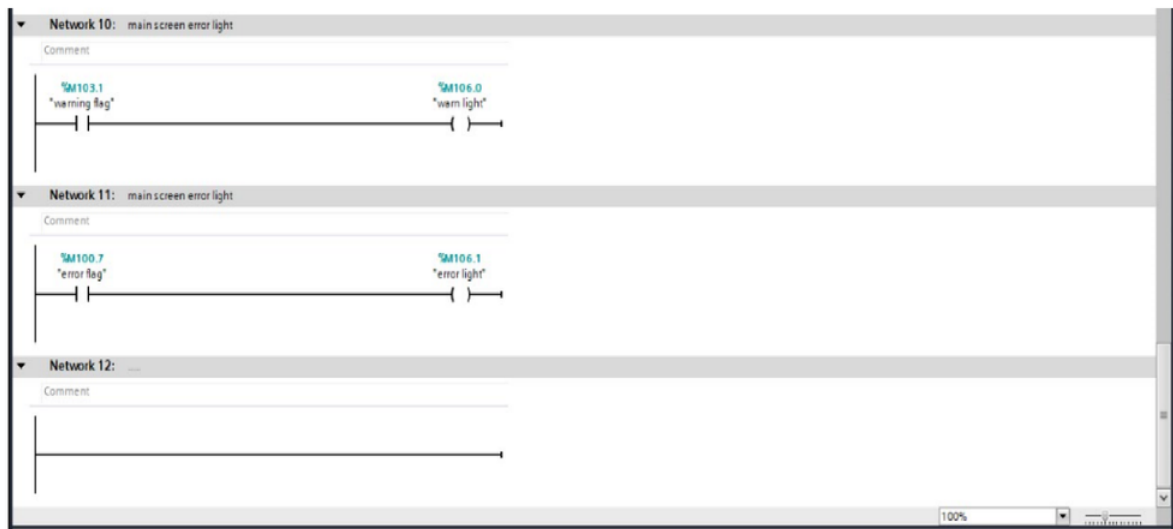
Figure 13. Networks 10 and 11 of the ladder logic program.
