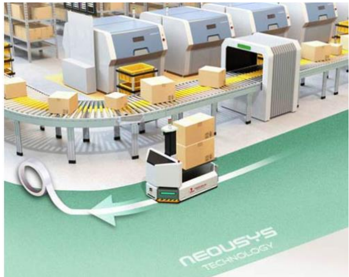
Figure 7 – Magnetic Tape guidance system
