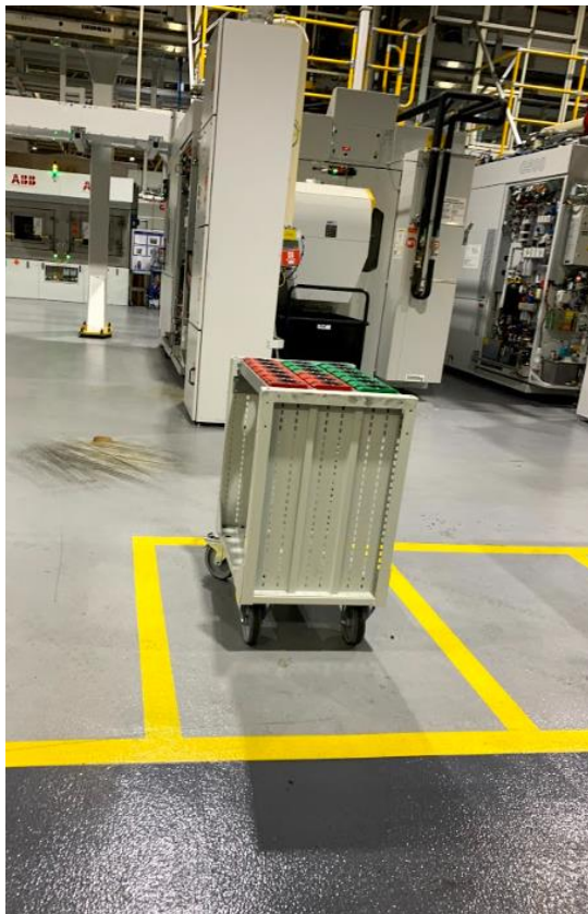
Figure 33 – Potential tool trolley drop off bays
