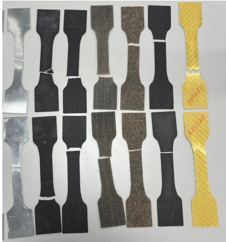
Figure 5 - Materials post failure left to right: Aluminium 1050 (assumed), Carbon Fibre non-woven mat Bio resin, Carbon Fibre woven Bio resin, Flax woven Bio resin, Flax non-woven Bio resin, Carbon Fibre woven Epoxy resin, Kevlar.
