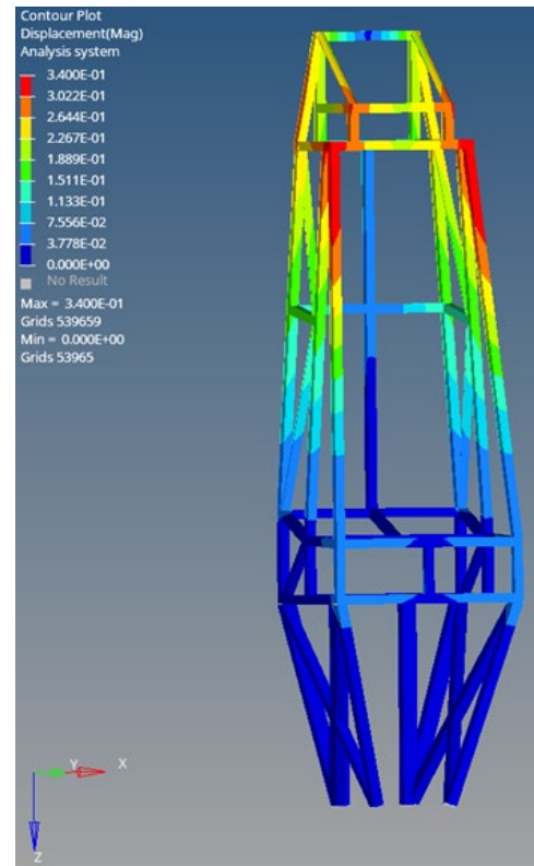
Figure-12 Result of FEA displacement simulation
