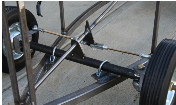
Figure 5.2: A traditional soapbox steering system (GordsGarage Blog, 2011)
