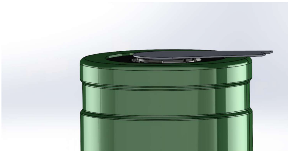
Figure 14. Solidworks model between the top (+ve) negative spring and the head of the cyclinder cell
